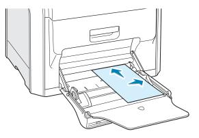
2 Pinch the paper width guide and slide it to the right to touch lightly against the edge of the paper without bending it.
